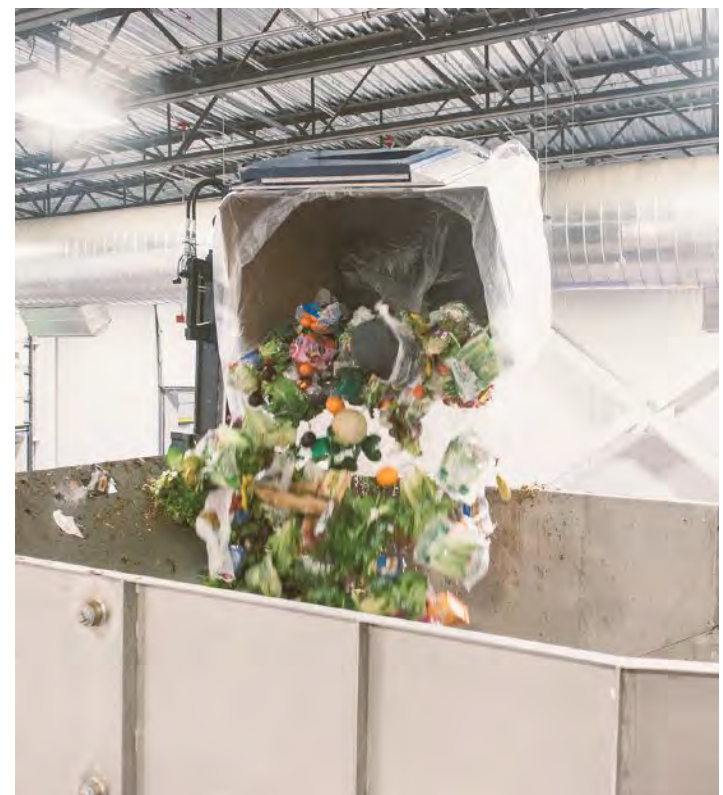
At left, Montague Transfer Station's compost program, where residents deposit food and paper waste; At right, At the Stop & Shop warehouse in Freetown, MA, food waste is emptied into a depackaging machine that separates food waste from packaging. The resulting food waste slurry is fed into the anaerobic digester that supplies power to the warehouse. (Image: Stop & Shop)
